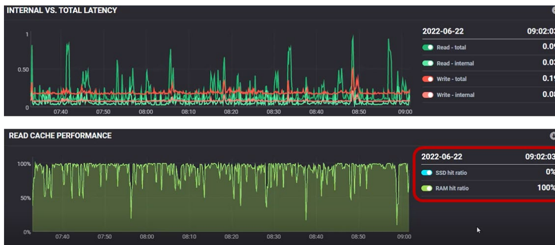
Figure 4. Read Cache Performance Observed on InfiniBox SSA II in Live Fortune 100 Environment
