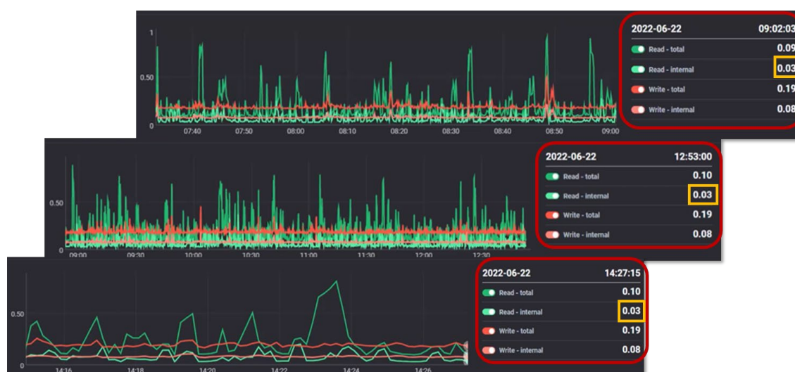
Figure 3. Storage Latencies Observed on InfiniBox SSA II in Live Fortune 100 Environment
