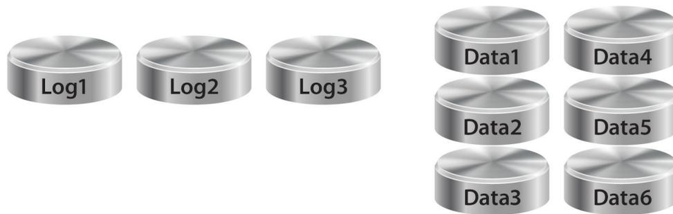
The figure above shows an example of a simplified Oracle data layout using a small number of equal-sized large LUNs for data, and one separate LUN for each of the redo log groups. In this example, a single Oracle data disk group using Oracle ASM can be created with the six larger LUNs, while three individual Oracle ASM disk groups can be created from the three smaller LUNs.
